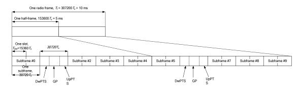
Figure 4.2-1: Frame structure type 2
