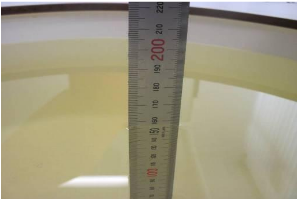
Picture 7-2: Liquid depth in the Flat Phantom (1800MHz)
