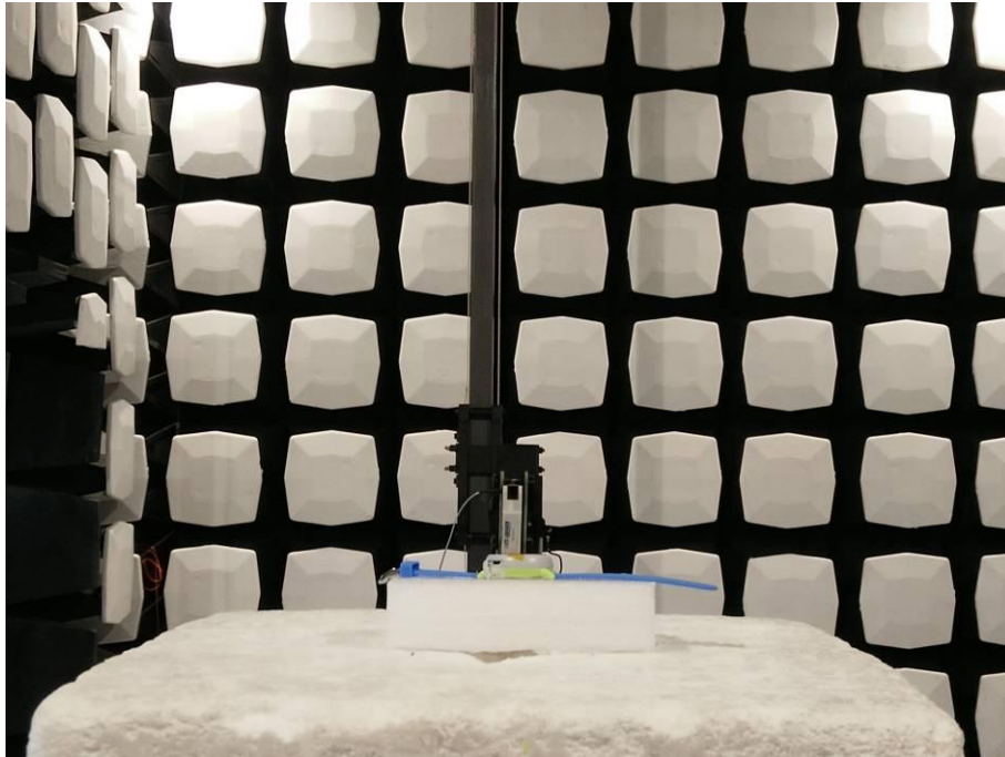
9. Radiated Emissions (Part 22/24) (Above 18GHz)
