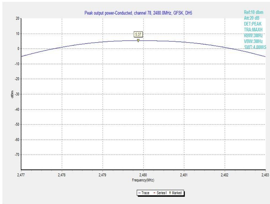
Fig. 3 Maximum Peak Output Power(GFSK, Ch 78)
