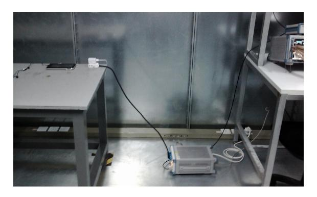
Radiation Emission Test Setup Below 1GHz
