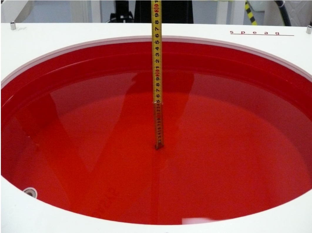
Picture 2: Liquid depth in the Flat Phantom (835 MHz, 15.1cm depth)
