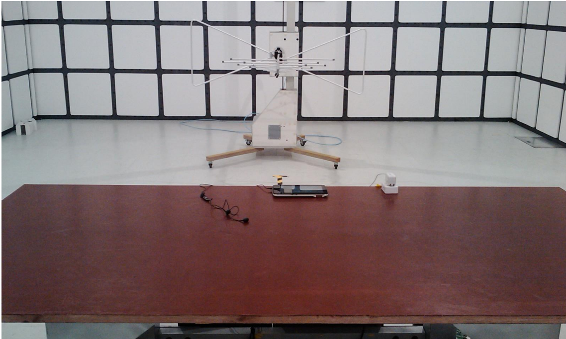
Radiated emission Test Set-up Front View
