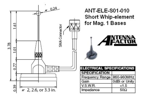
The coaxial cable length is set to 10 feet.
