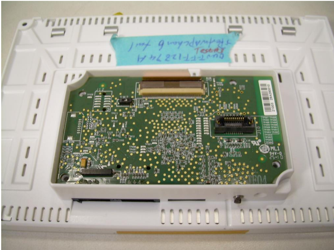
Photograph 15 – View of the Interface Side of the Display PCB
