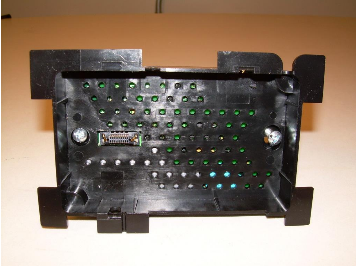
Photograph 14 – View of the Power Supply/Interface Module with Display Removed
