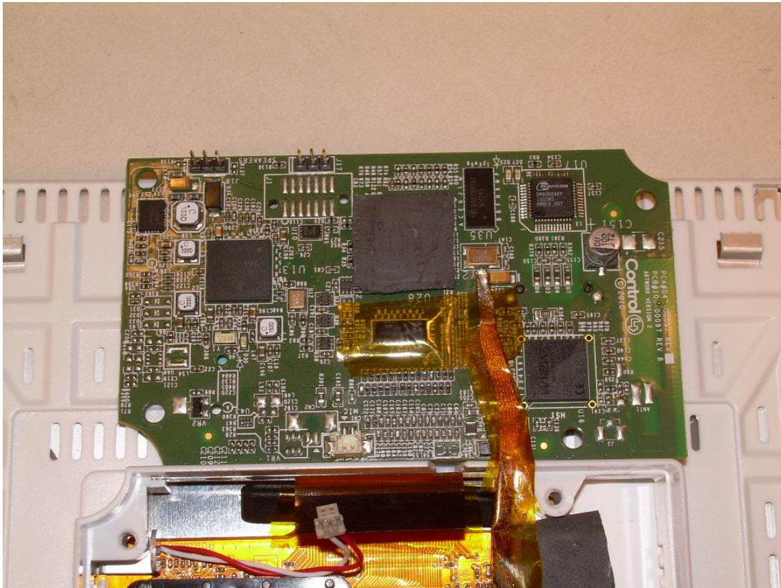
Photograph 16 – View of the Component Side of the Display PCB showing Ferrite on Flex Cable
