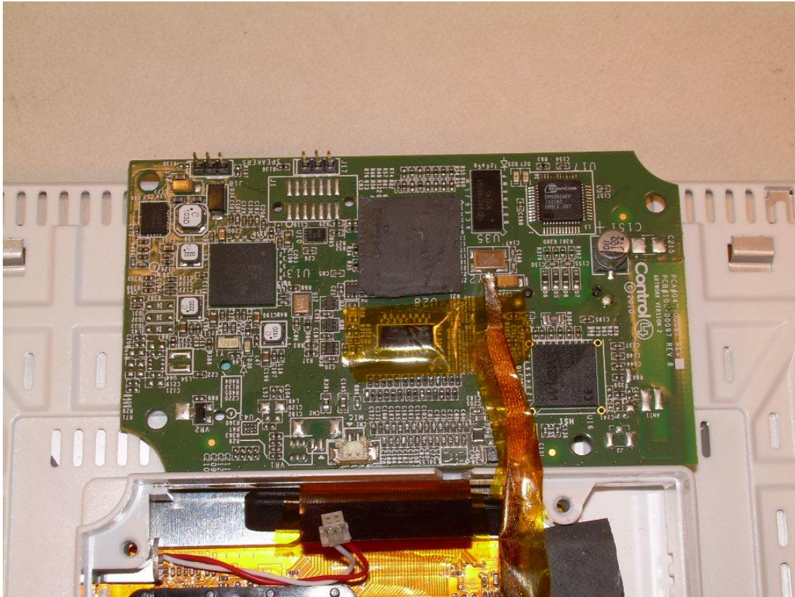
View of the Component Side of the Display PCB showing Ferrite on Flex Cable
