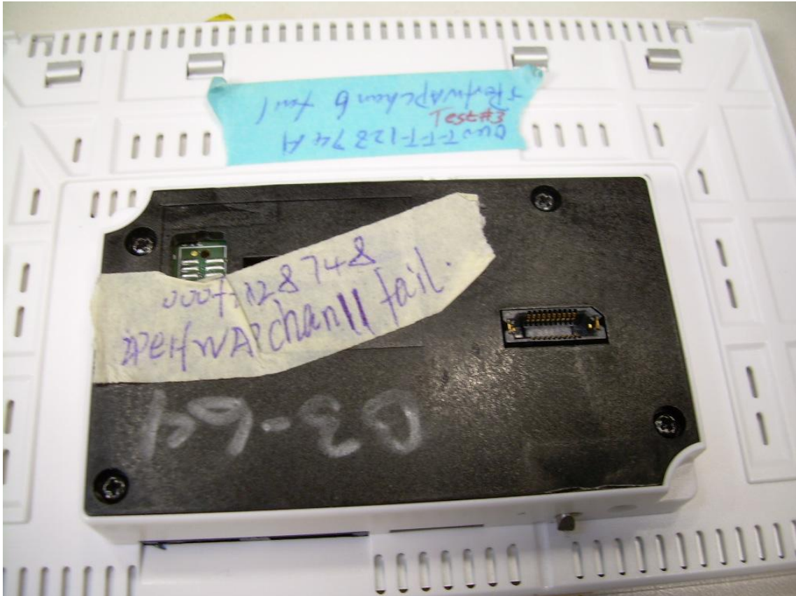
Back View of the Display Separated from Power Supply/Interface Module
