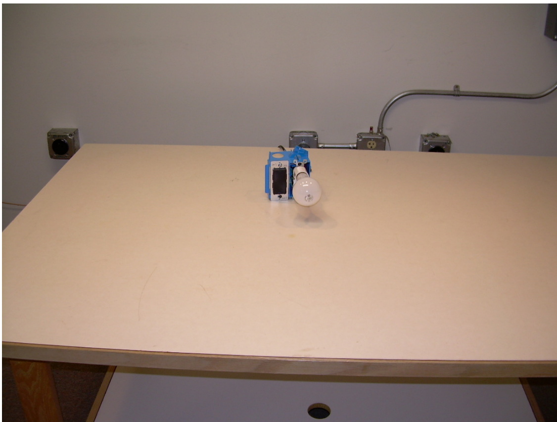
Photograph 3 - Front View Conducted Disturbance Worst Case Configuration
