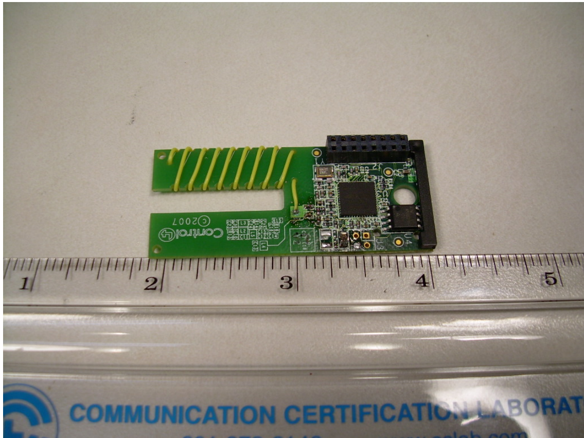
Photograph 10 - Back View of the Transceiver PCB
