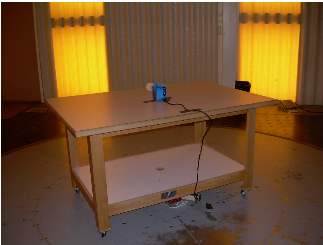
Photograph 2 - Back View Radiated Spurious Emission Test Configuration
