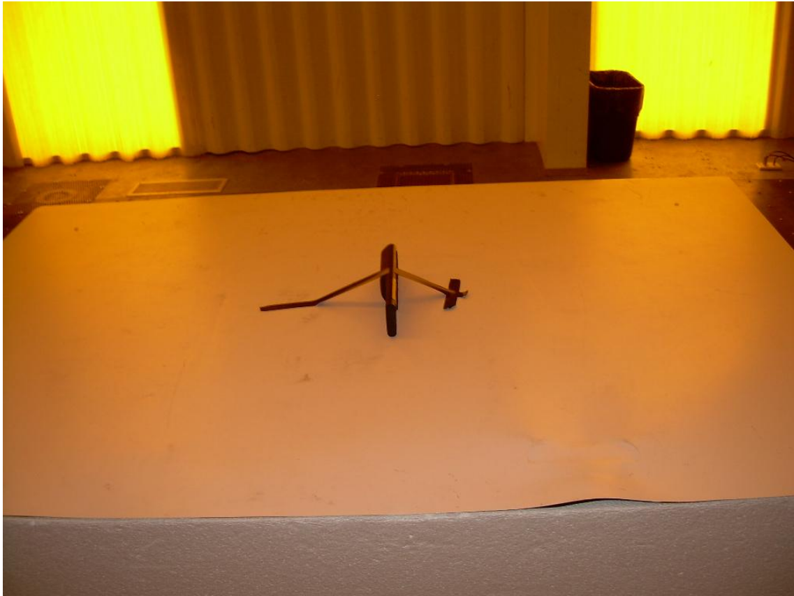
View of Radiated Emission Setup – On Edge EUT Placement
