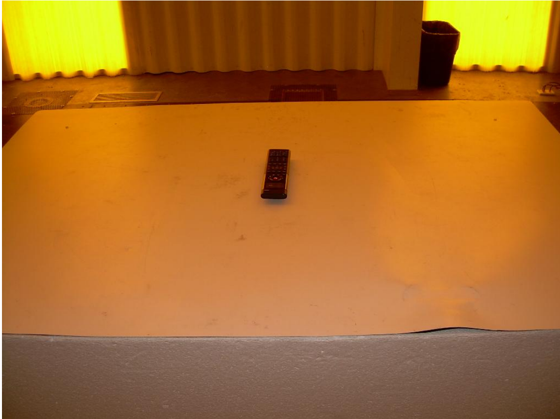
Photograph 3 – View of Radiated Emission Setup – Horizontal EUT Placement
