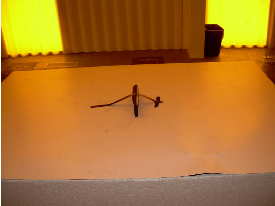
Photograph 2 – View of Radiated Emission Setup – On Edge EUT Placement
