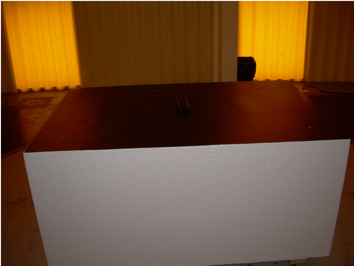
Photograph 1 - Radiated Emission Test Setup - Horizontal Placement
