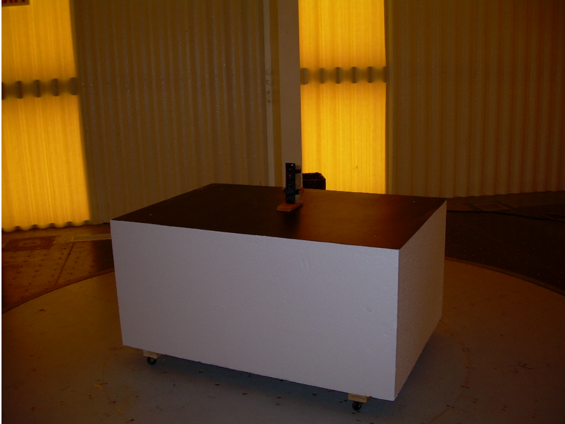
Photograph 2 - Radiated Emission Test Setup - Vertical Placement
