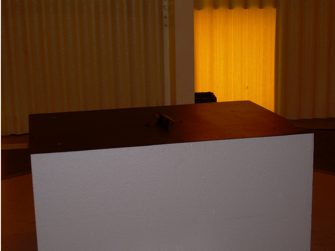
Photograph 3 - Radiated Emission Test Setup - On-edge Placement
