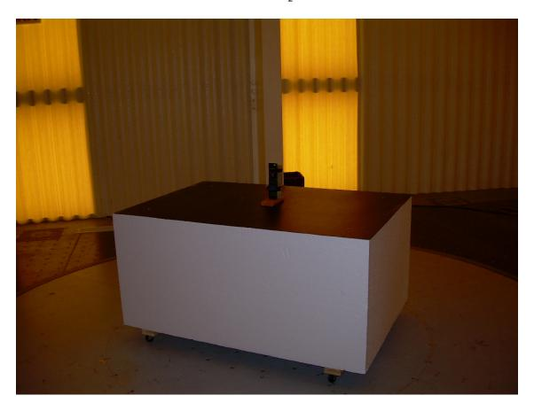
Radiated Emission Test Setup - On-edge Placement
