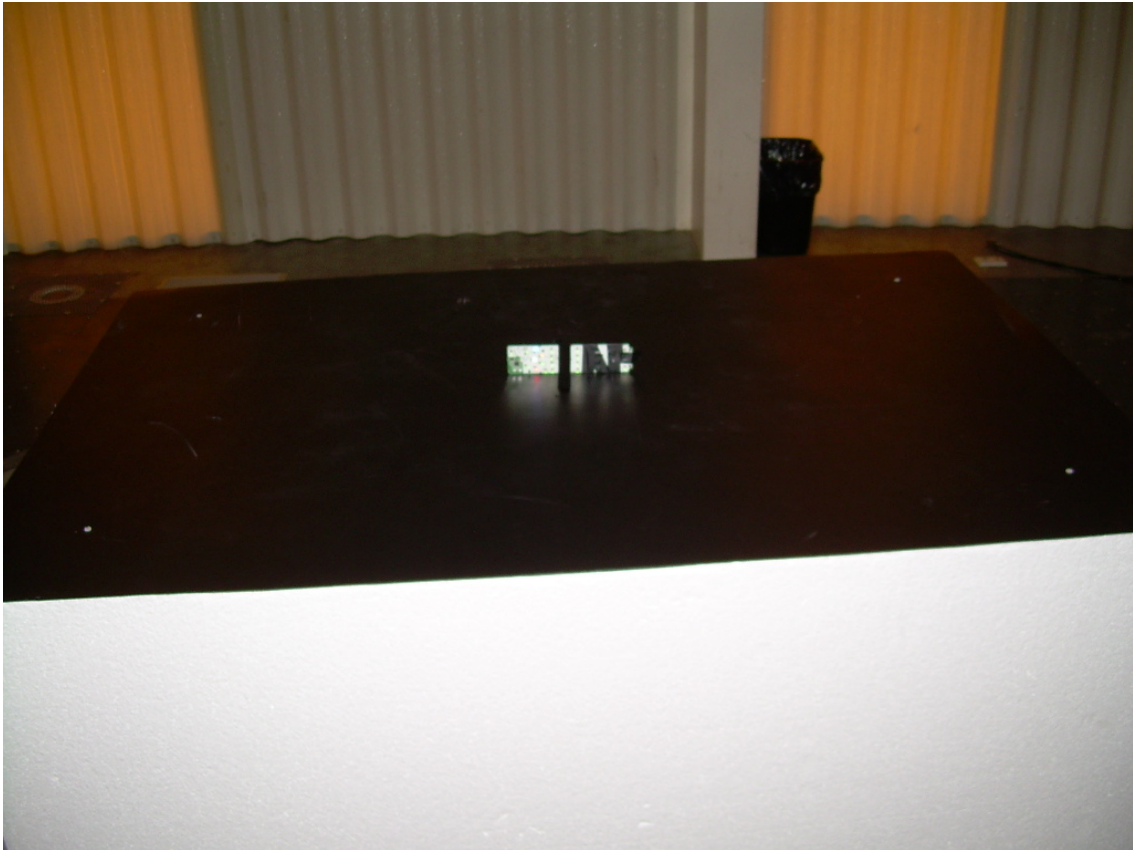
Photograph 2 - Radiated Spurious Emission Test Setup - On Edge Placement
