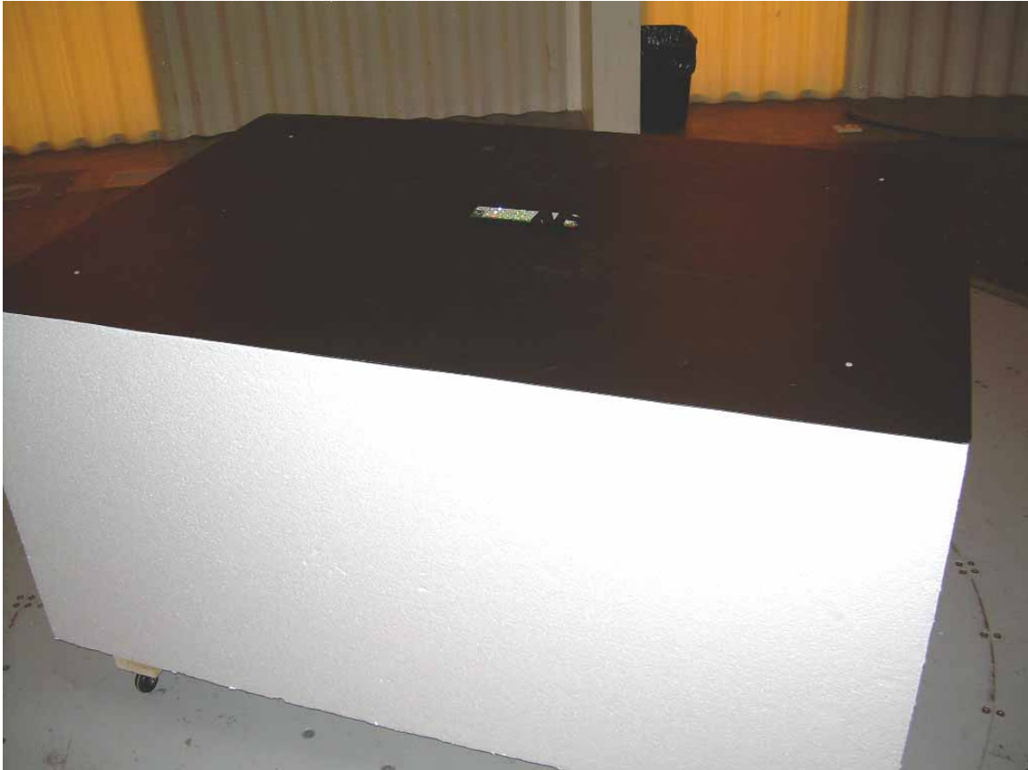
Photograph 1 - Radiated Spurious Emission Test Setup - Horizontal Placement
