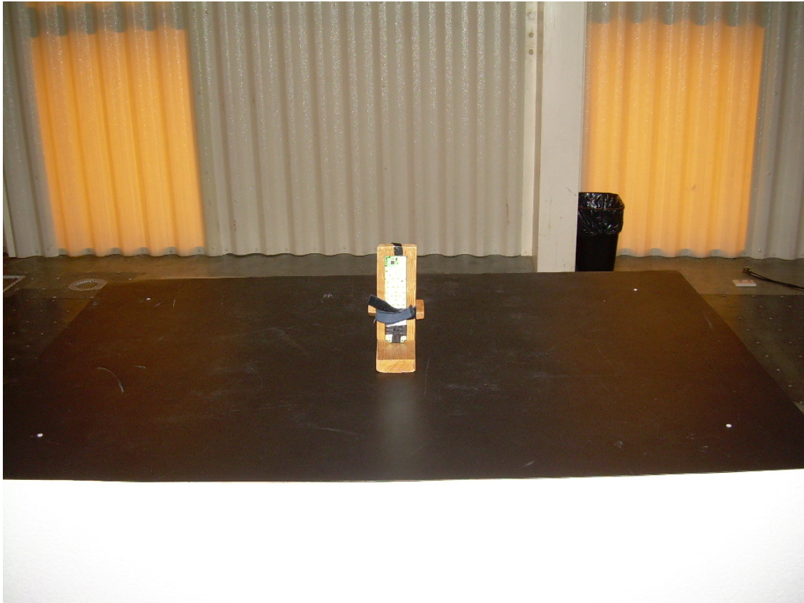
Photograph 3 - Radiated Spurious Emission Test Setup - Vertical Placement
