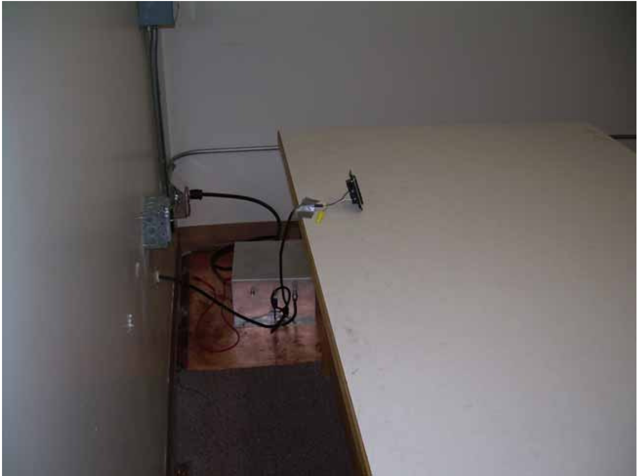
Back View Conducted Disturbance Worst Case Configuration
