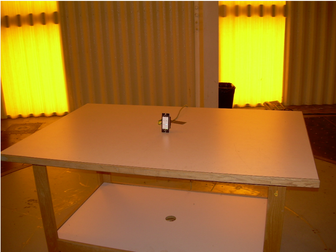
Photograph 1 - Front View Radiated Spurious Emission Test Configuration
