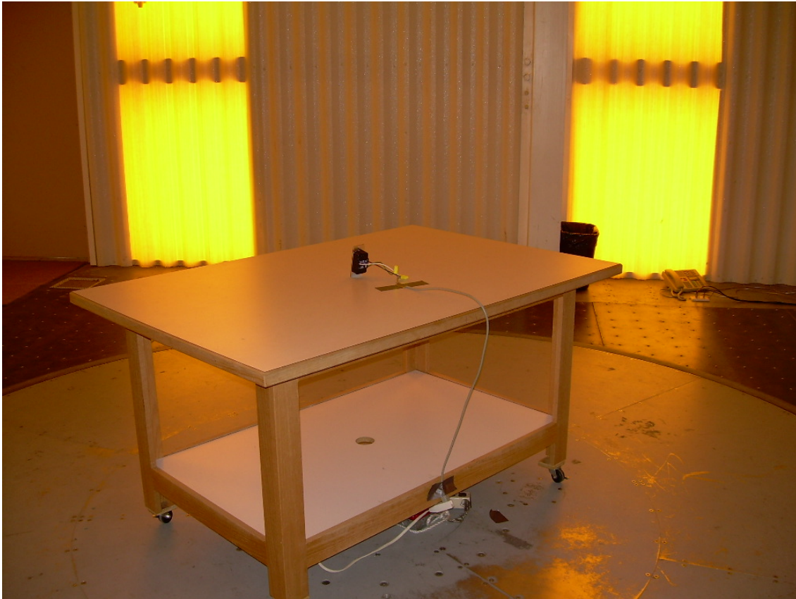
Photograph 2 - Back View Radiated Spurious Emission Test Configuration
