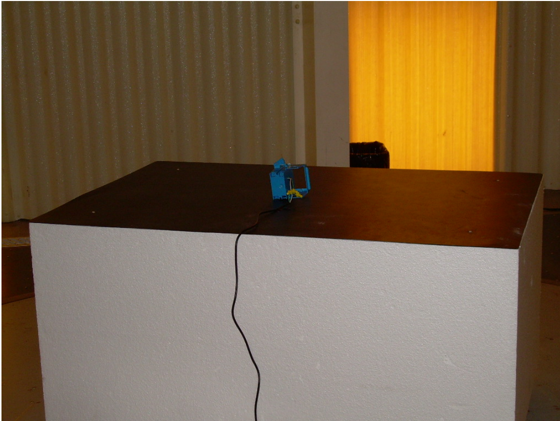
Photograph 2 - Back View Radiated Emissions in the Restricted Bands - Worst Case Configuration
