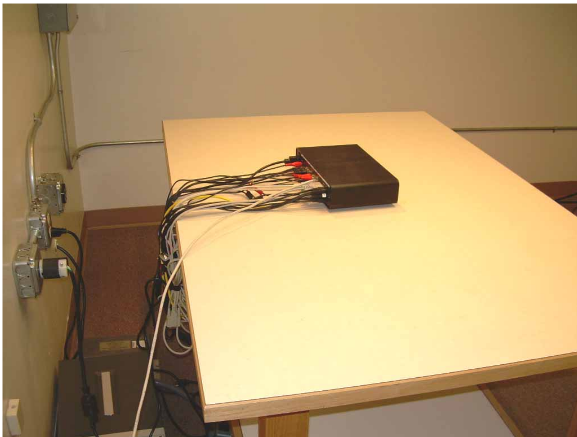
Photograph 4 - Back View Conducted Disturbance Worst Case Configuration
