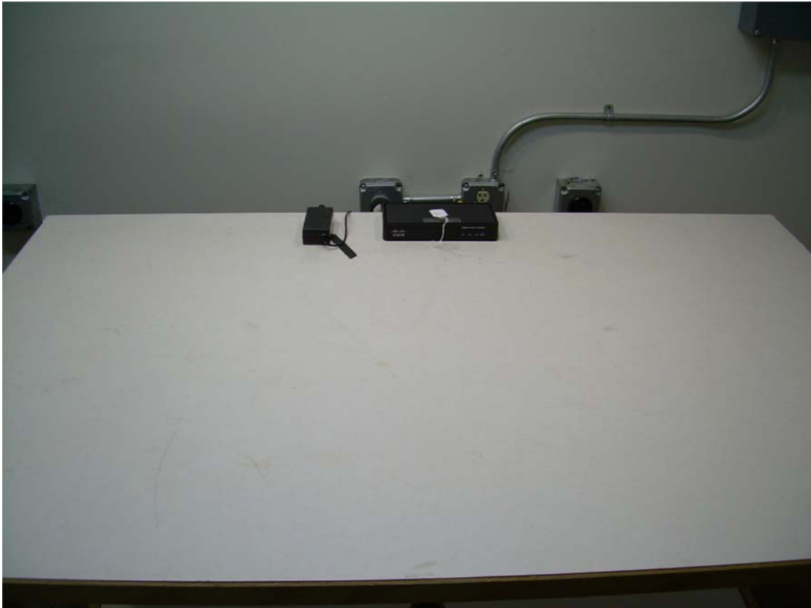
Front View Conducted Disturbance Worst Case Configuration
