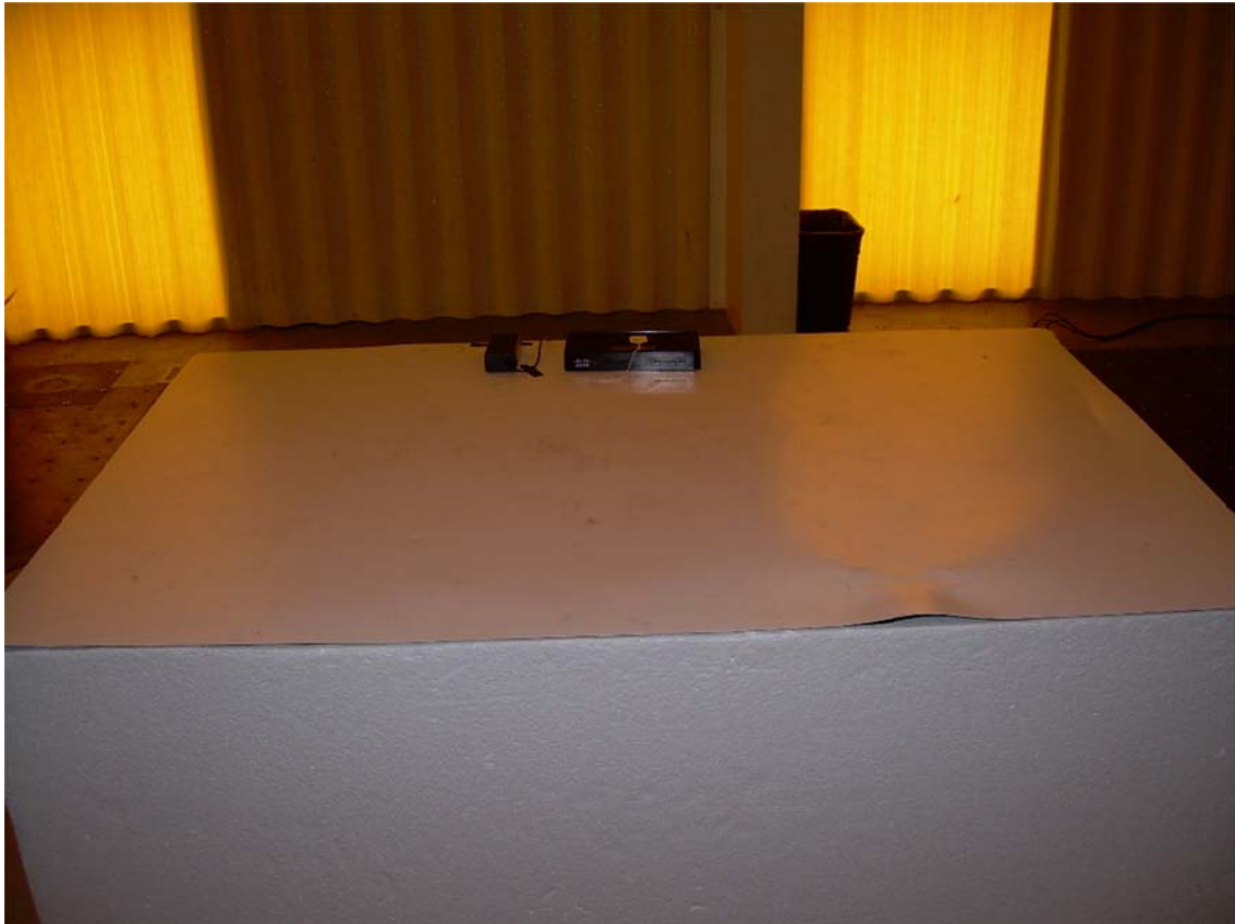
Front View Radiated Disturbance Worst Case Configuration
