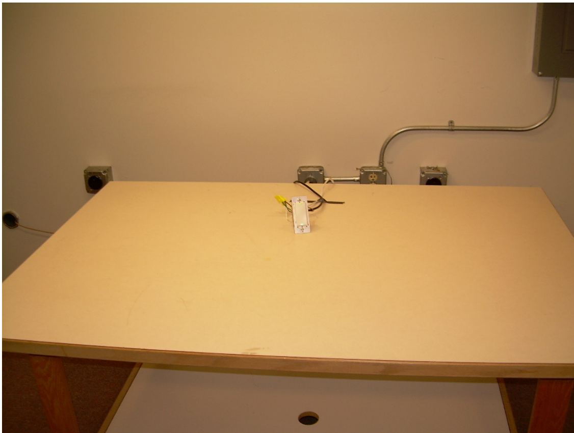
Photograph 3 - Front View Conducted Disturbance Worst Case Configuration
