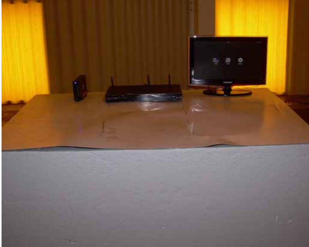
Photograph 1 – Front View of the Radiated Emission Setup
