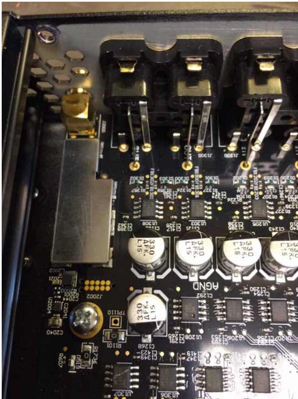
Photograph 9 – View of the 802.15.4 Transceiver Circuitry with RF Shield
