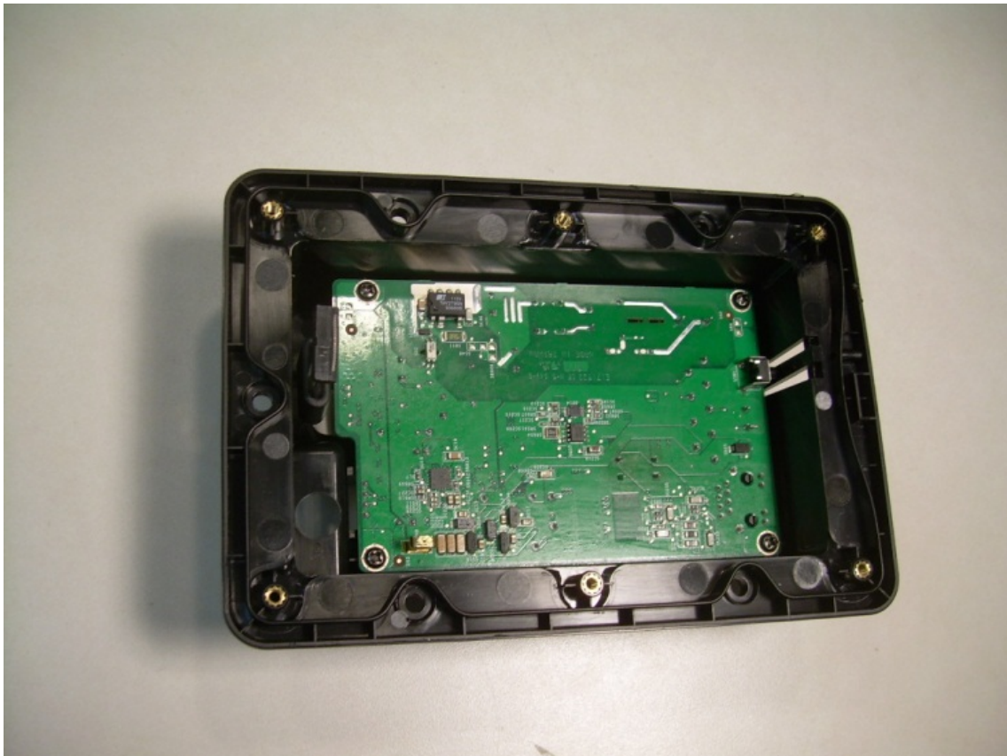
Photograph 18 – View of the EUT Inside Back Housing Showing the Power PCB Placement
