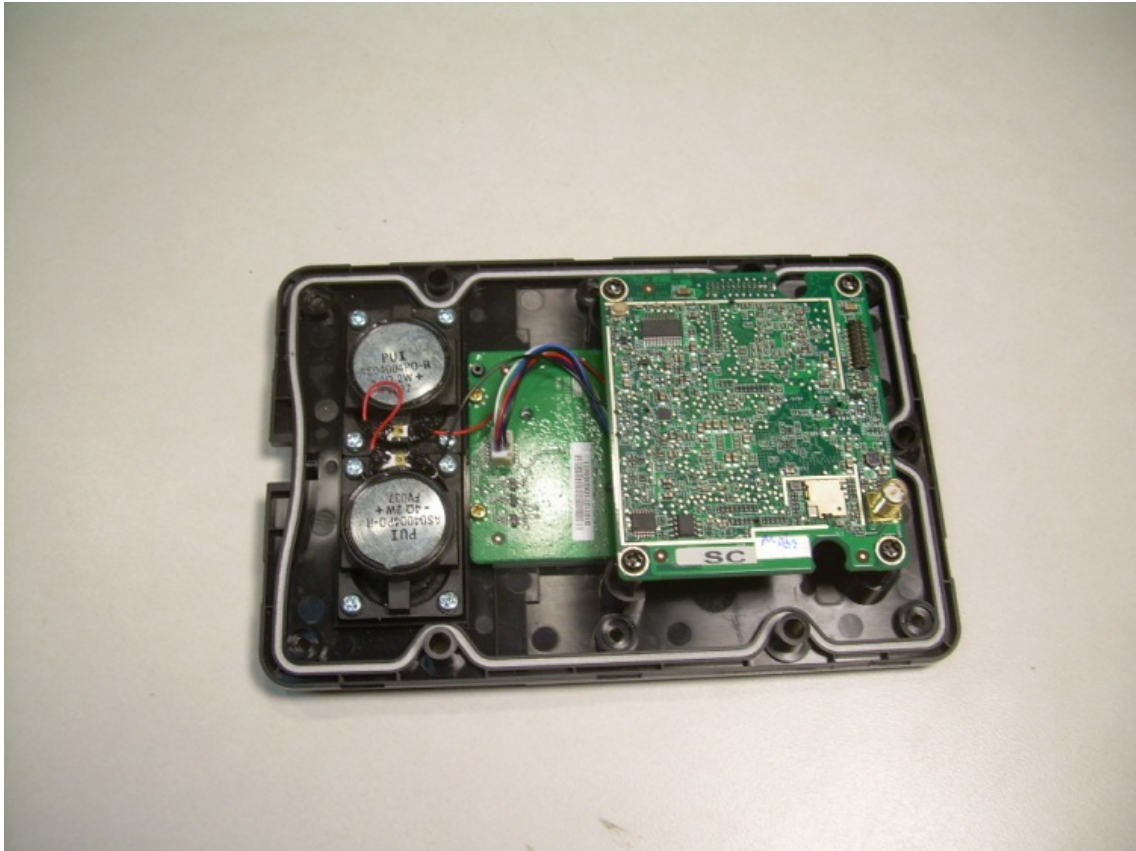
Photograph 21 – View of the Front EUT Housing Showing Main/RF PCB and Switch PCB
