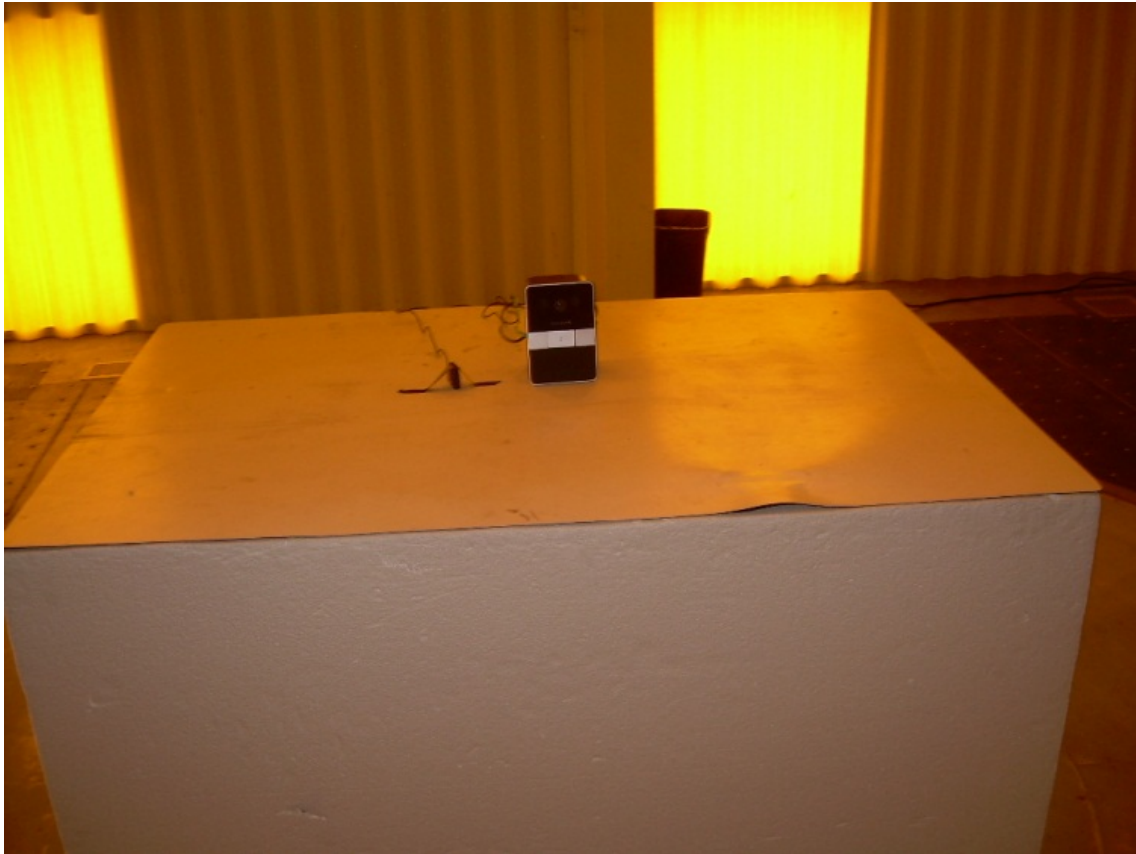
Front View Showing Worst-Case Patch Antenna Placement
