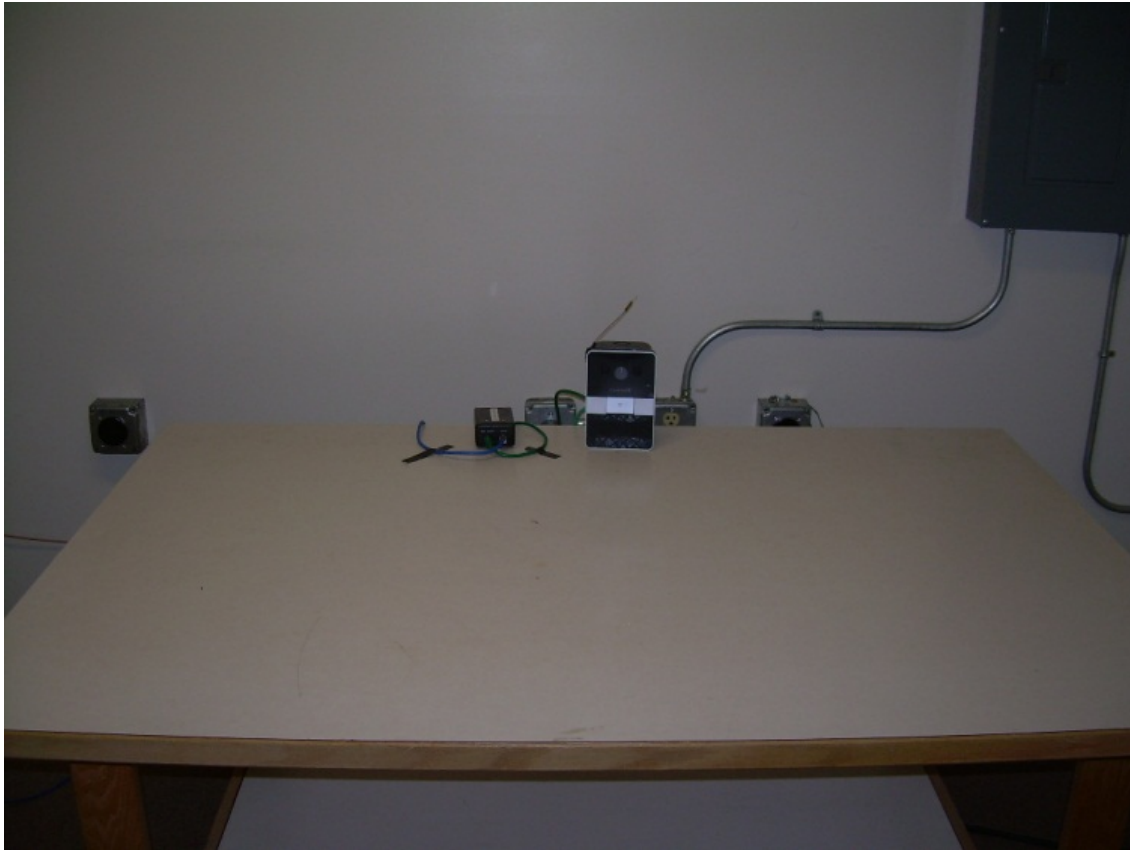
Front View Conducted Disturbance Worst Case Configuration – POE Power
