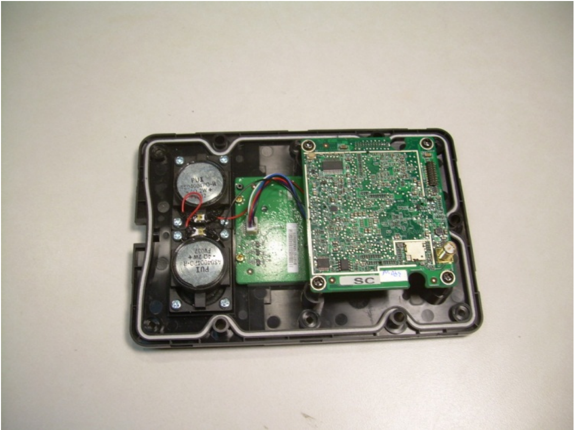
View of the Front EUT Housing Showing Main/RF PCB and Switch PCB
