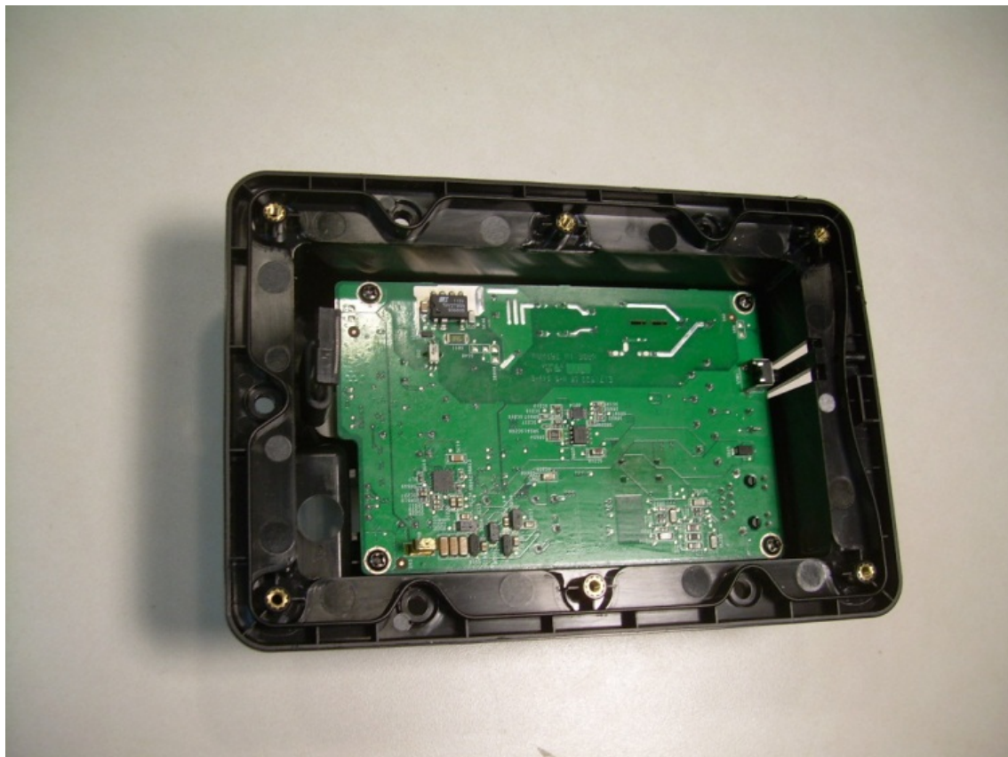
View of the EUT Inside Back Housing Showing the Power PCB Placement
