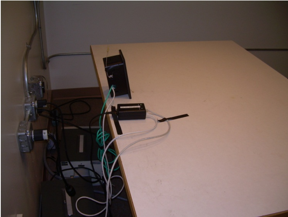
Photograph 9 – Back View Conducted Disturbance Worst Case Configuration – POE Power
