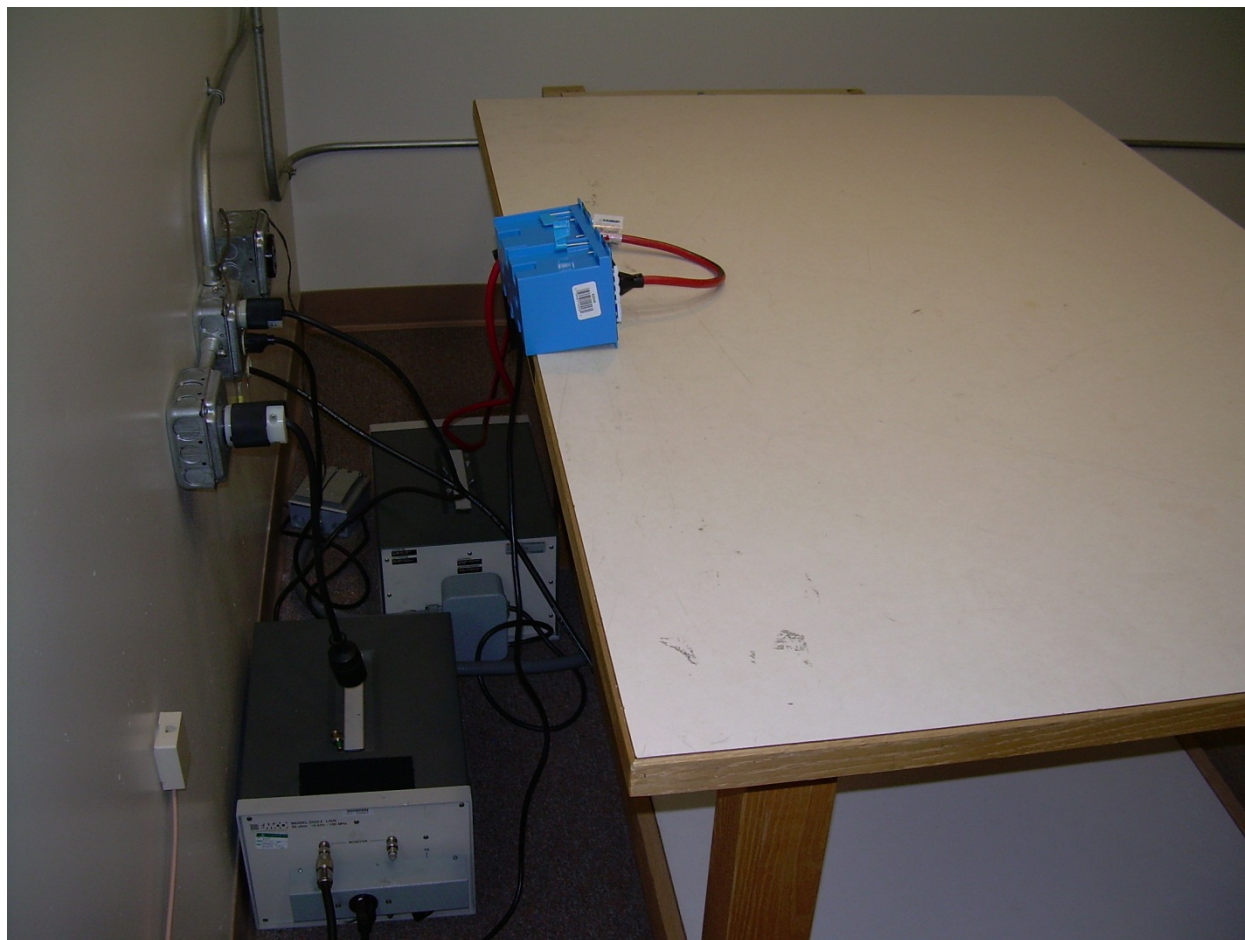
Photograph 4 – Back View Conducted Disturbance Worst Case Configuration
