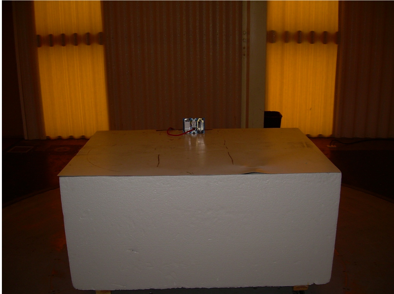
Photograph 1 – Front View Radiated Disturbance Worst Case Configuration
