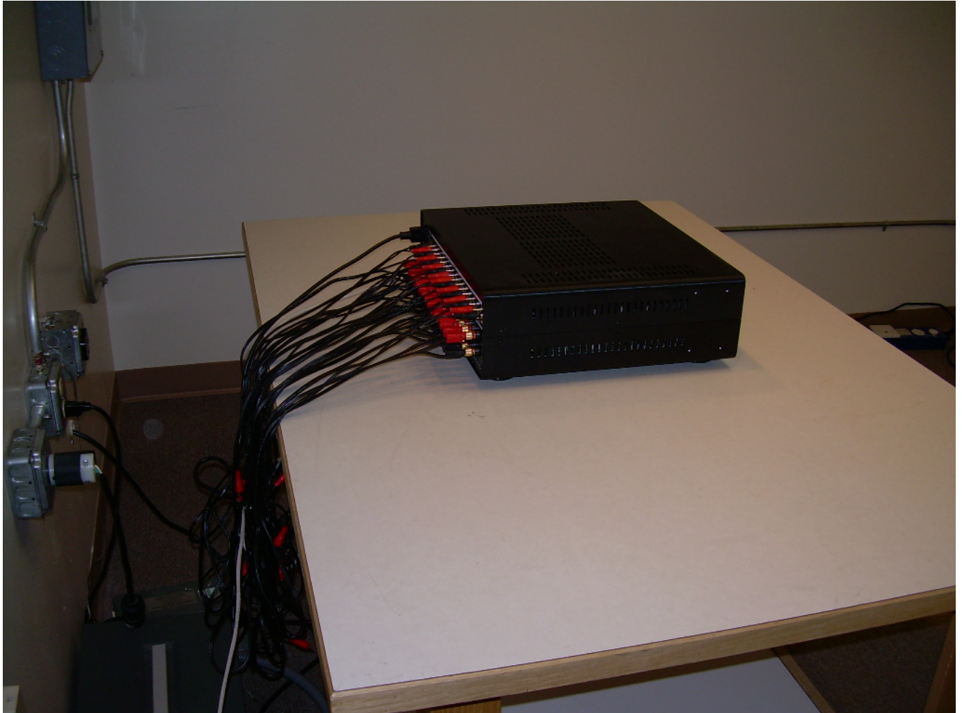
Photograph 4 - Back View Conducted Disturbance Worst Case Configuration
