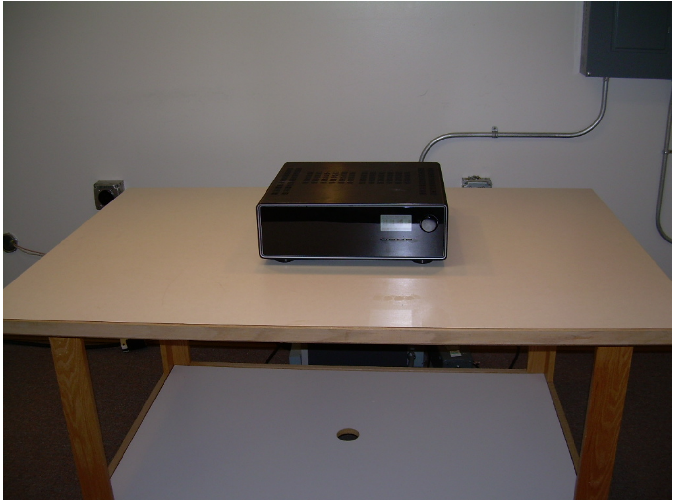
Photograph 3 - Front View Conducted Disturbance Worst Case Configuration
