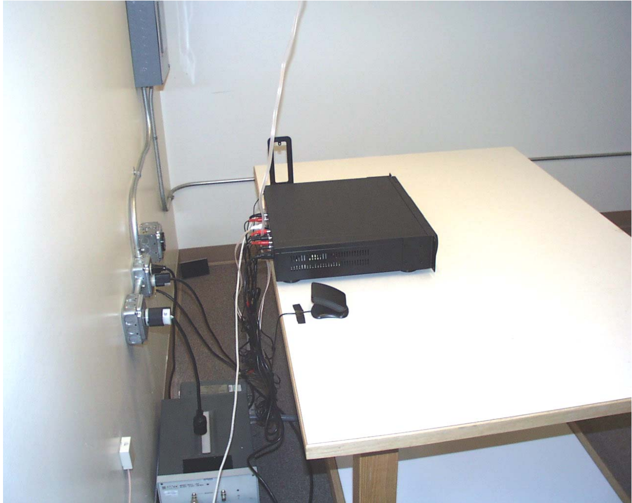
Photograph 4 - Back View Conducted Disturbance Worst Case Configuration
