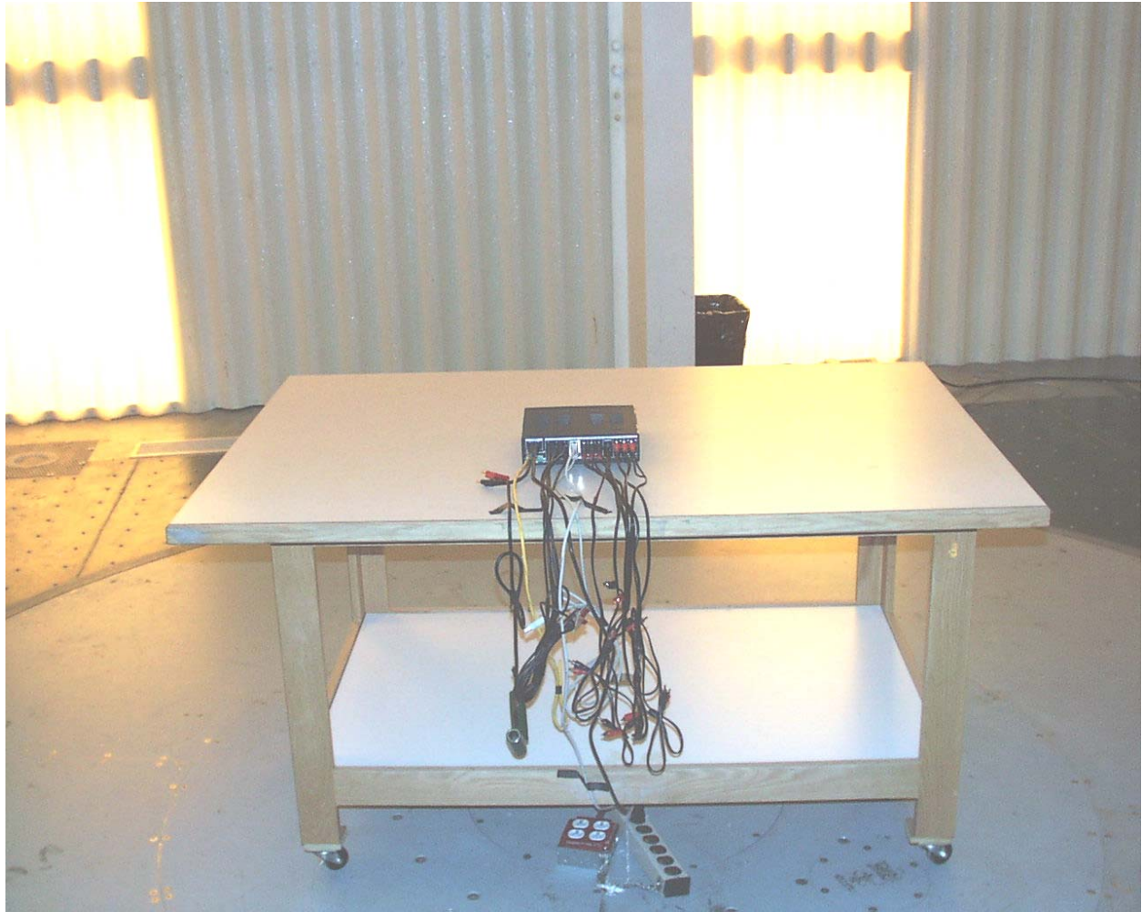
Photograph 2 - Back View Spurious Radiated Emission Worst Case Configuration
