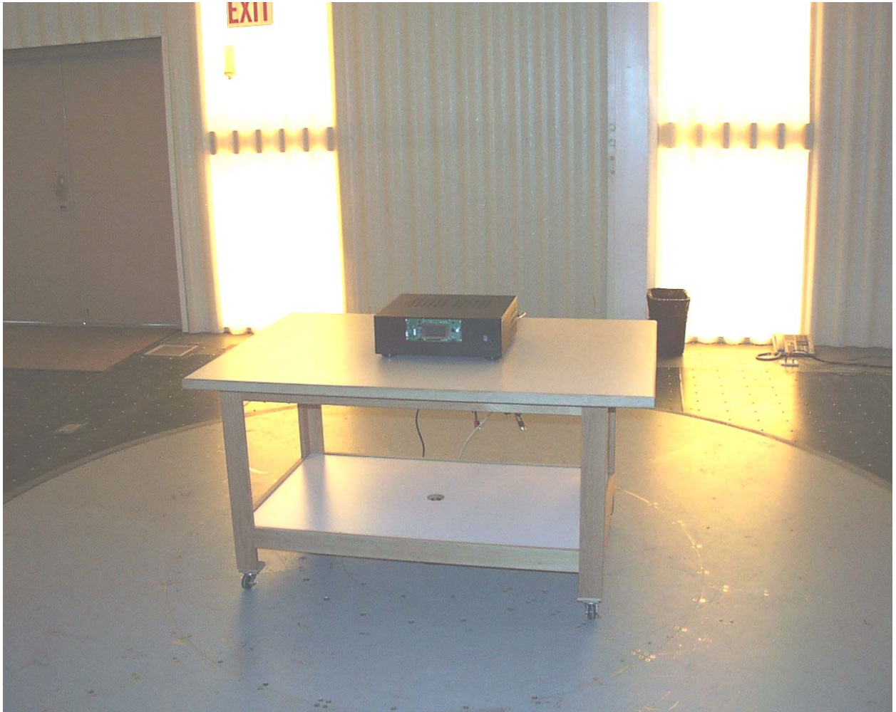
Front View Radiated Disturbance Worst Case Configuration
