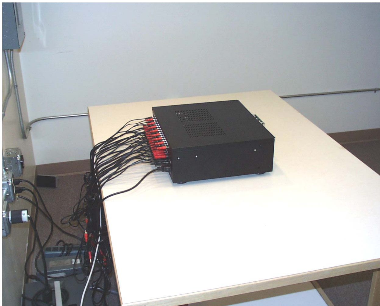
Photograph 4 - Back View Conducted Disturbance Worst Case Configuration
