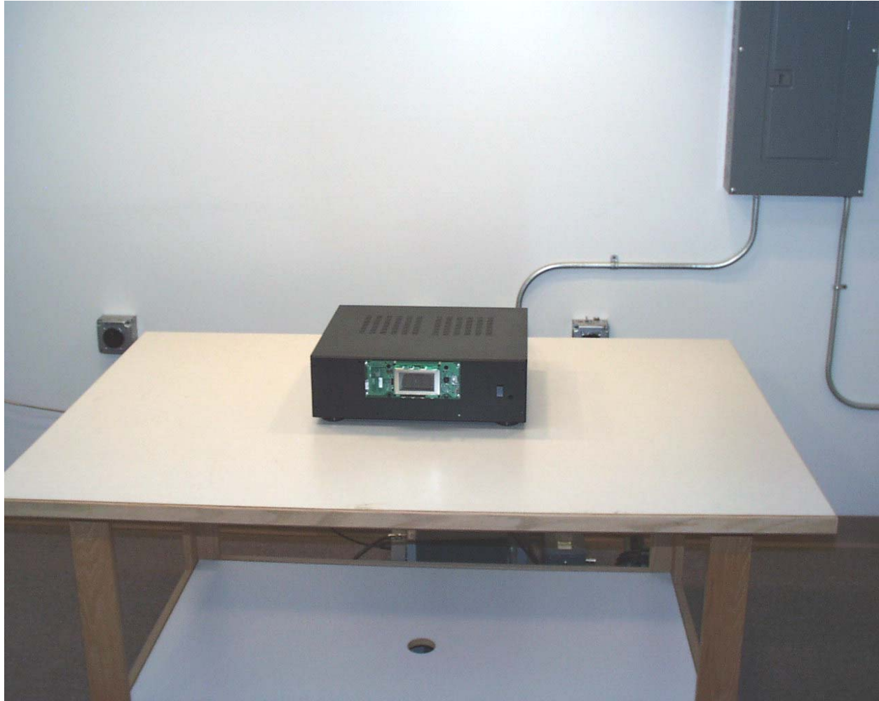
Photograph 3 - Front View Conducted Disturbance Worst Case Configuration
