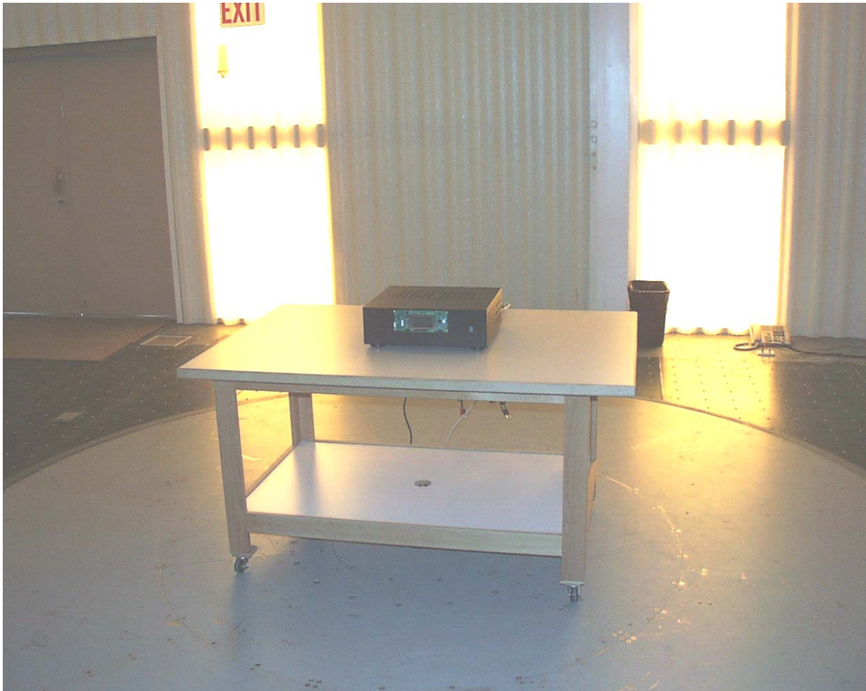
Photograph 1 - Front View Radiated Disturbance Worst Case Configuration
