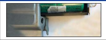
2. Attach the Power Adaptor to the connector plug. As soon as you plug the adaptor into the lock, it will cycle until it is ready to open.
