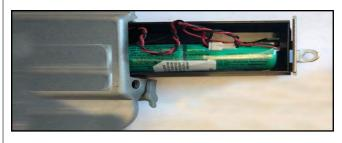
4. The lock should be available for installation about 10 seconds after battery installation.
