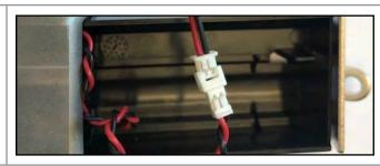
3. Place the battery into the battery compartment, carefully tucking wire in before closing compartment.
