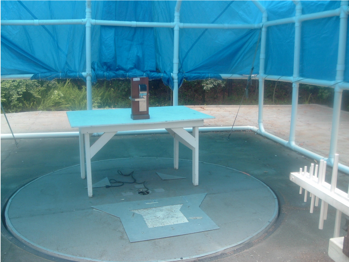
Figure 4. Front View of EUT (radiated emissions testing)
