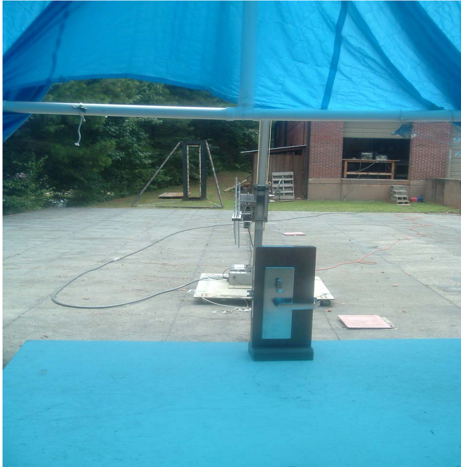
Figure 5. Rear View of EUT (radiated emissions testing)
