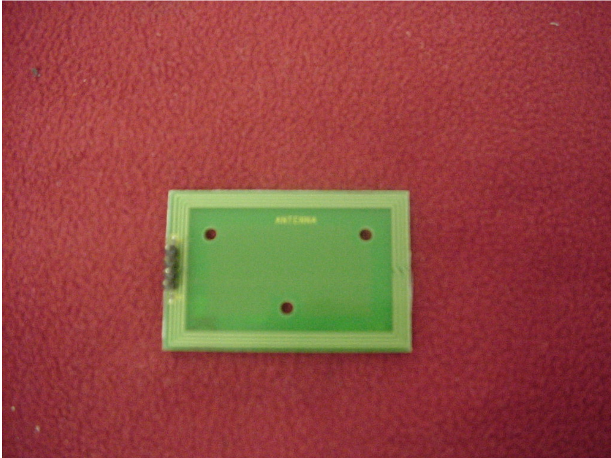
Photo 5. Antenna Board, Antenna Side
