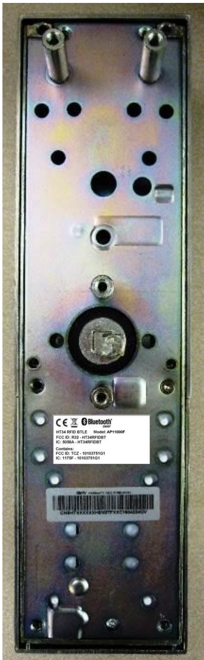
Figure 1. Location of labeling on the back side of the assembled HT RFID.
