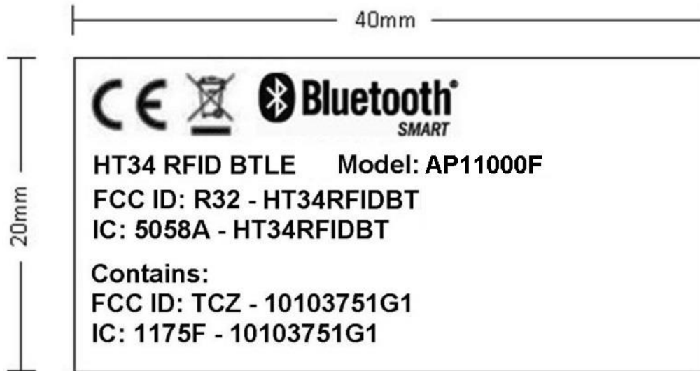
Figure 2. Approximate design of the label applied to the assembled HT RFID chassis.
