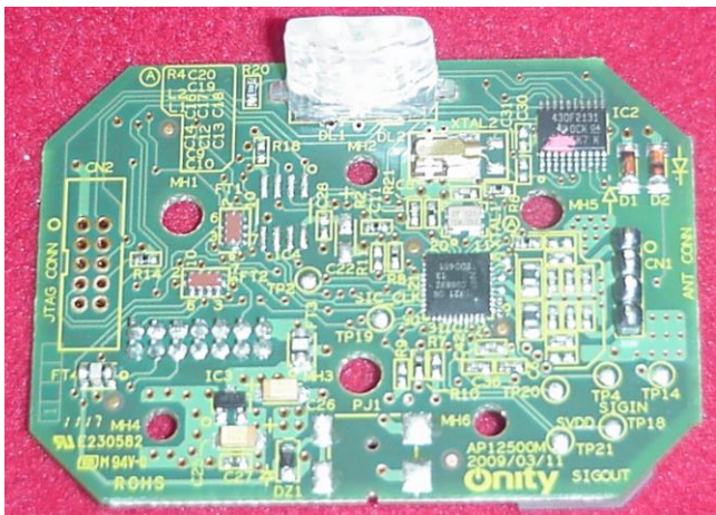
Figure 5. Top view of the RH's RFID reader PCB.
