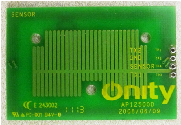
Figure 3. Top view of the RH's antenna PCB.
