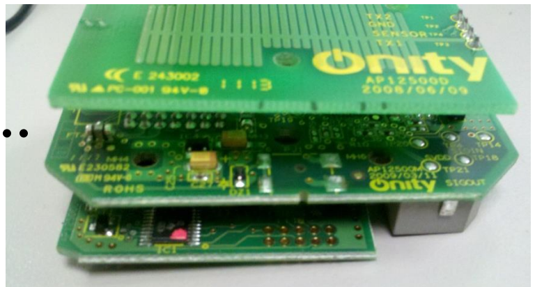
Figure 2. The three PCBs contained inside the HT34's RH.
