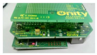
Figure 2. The three PCBs contained inside the ADVWR RH.
