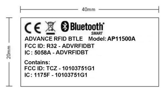
Figure 2. General layout and dimensions appearing on the ADV label.
