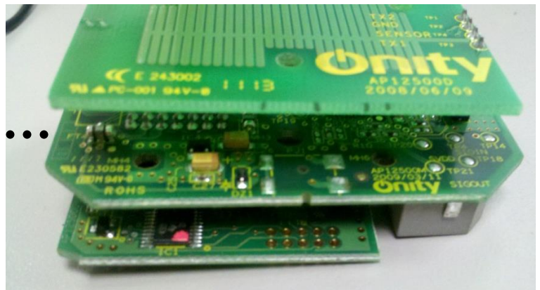
Figure 2. Three PCBs contained inside the RH.
