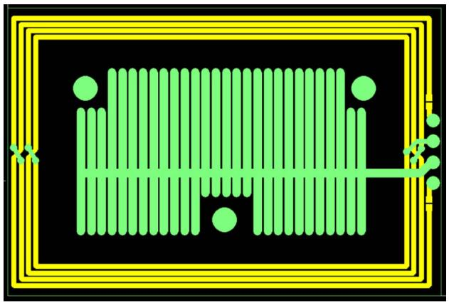
Figure 1. The PCB layout of the RFID antenna.
