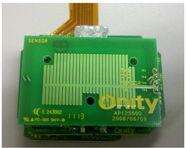
Figure 2. The RFID antenna mounted to the top of its other RFID PCBs.
