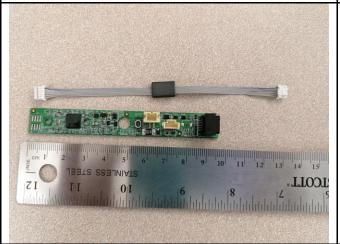
Motor Board Front View and Cable Connector
