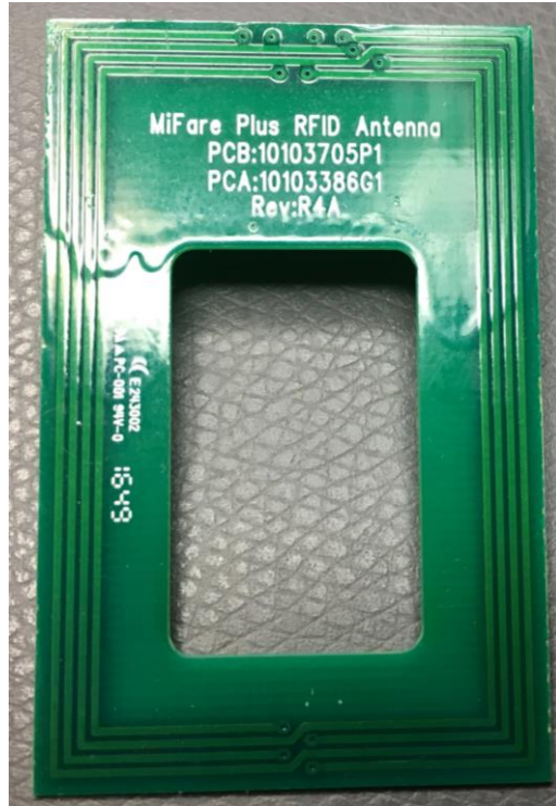
Figure 3. Top view of the RH's antenna PCB.
