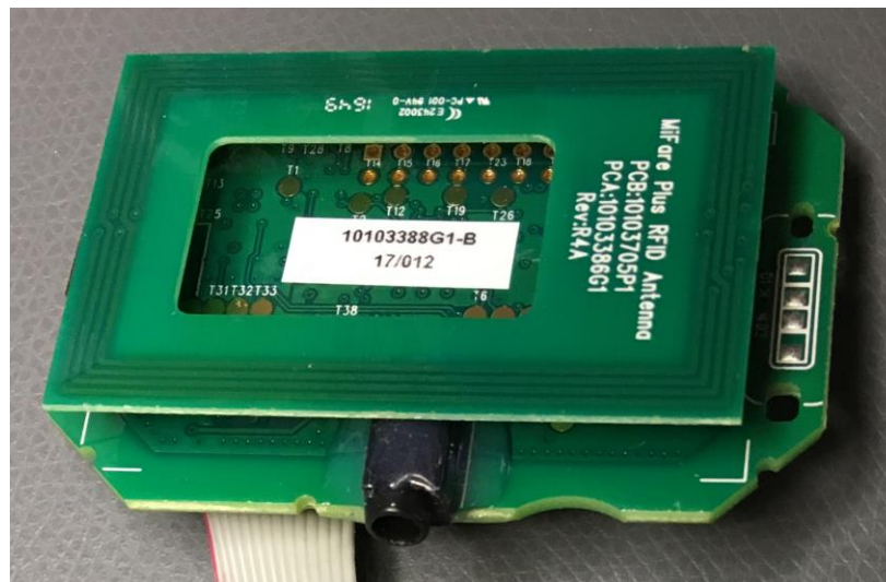
Figure 2. The two PCBs contained inside the OS700 Safe for reading key cards – bottom view.
