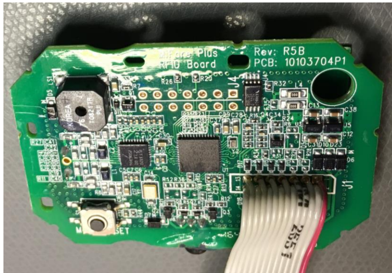
Figure 1. The safe's assembled RFID Read Head – top view.
