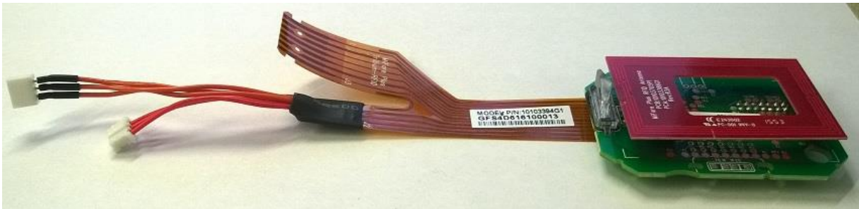
RFID reader circuit assembly (three circuit boards, soldered together), top
