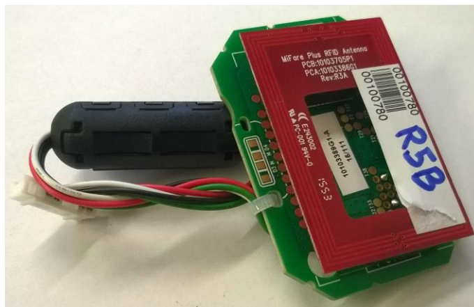
RFID reader circuit assembly (two circuit boards, soldered together), top
