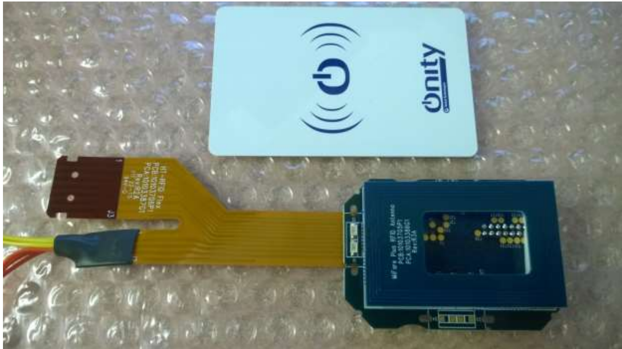
Figure 2. RFID Reader electrical assembly (with antenna), with standard RFID card
