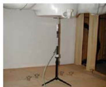
Figure 15.1 Dipole Validation Test Setup
