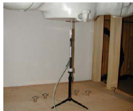
Figure 12.1 Dipole Validation Test Setup
