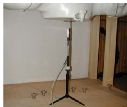
Figure 12.1 Dipole Validation Test Setup
