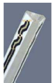
Figure 3.2 Probe Thick-Film Technique
